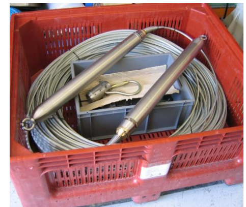
Two PSS tools complete with 200m cables, quick release cable clamp and T-bars in a custom transit basket.
