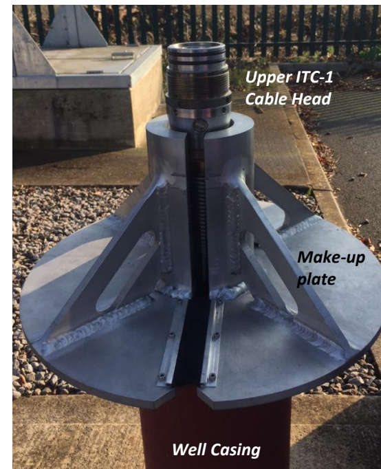
SMUP Example – used on well casing, ITC-1 cable suspended in well using make up plate.
