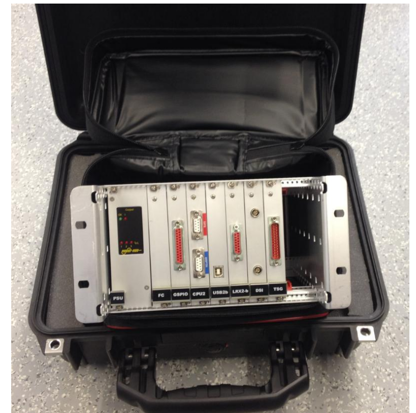
GSP Spares Kit in aluminium storage rack (27x13cm), shipped within protective bag and peli 1450 case
