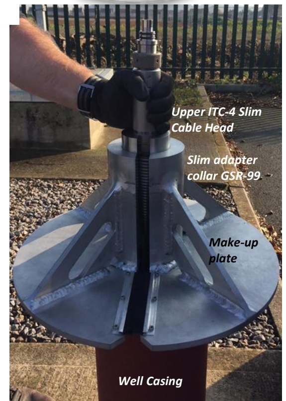
SMUP Example with slim adapter collar (GSR-99) – used on well casing, slim ITC-4 cable suspended in well using make up plate.
