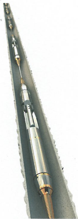
Figure 1. Downhole geophones with locking arm to couple to formations/casing.
